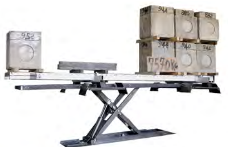
LOAD TEST ON WHEELS + 50% OVERLOAD EN 1493 EUROPEAN STANDARD 2 PORTIONS ON ONE SIDE 1 PORTION ON THE OPPOSITE SIDE
