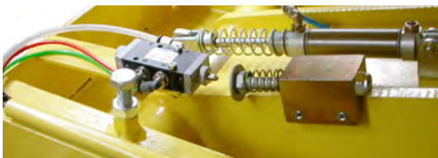
Safety device stopping the lift on getting out of the pit, against damage to the underside of a vehicle, and on getting into the pit (on PH and PE versions on getting out of the pit)
