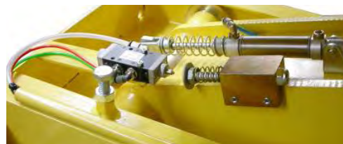
Safety device operating during lowering with acoustic signal activation (on JO.30JP and JO.35)
