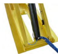
Safety device operating during lowering with acoustic signal activation
